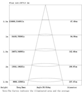
eline turves indicate the illuminated area and the average illumination when the luminaire is at different distance.
