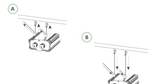
Lift the LED and attach the carabiners to pre-installed hooks from ceiling or mounting beam. The Ratchets should be installed closest to the LED (and not the ceiling).
