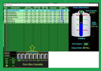
Tank levels are consistently visible while the system is running, in order to ensure that levels of all nutrients are being tracked. The Fertigation Manager Pro further offers the ability not only to monitor nutrient tanks, but also solutions within each tank. Changes can be easily configured to change levels per stroke, capacity, and alarm setpoints (based on percentage).
