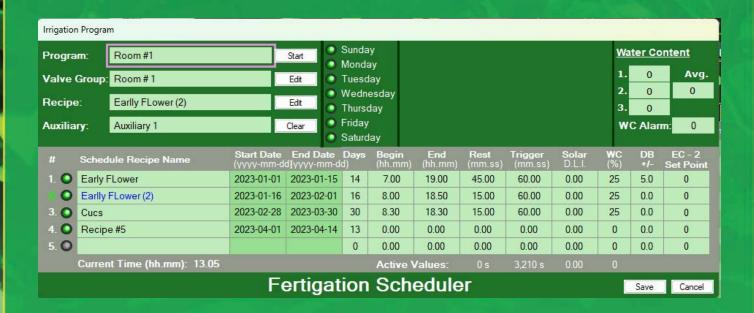
There are 20 irrigation programs where one can assign specific irrigation valves. Schedule irrigation based on time intervals, live solar conditions set in u/Moles, by substrate/soil moisture sensors or by external trigger.
