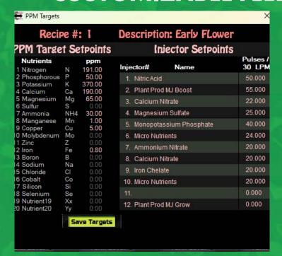
Get unprecedented control by specifying up to 150 different Feed Formulas, on 150 different schedules, controlling up to 150 valve groups, with EC control feed formulas for specific targeting. All formulas are based off of PPM measurements for more accurate formula integration, and feature integrated manual testing option before actioning them within a grow zone, ensuring accuracy for your formulas and schedules.
